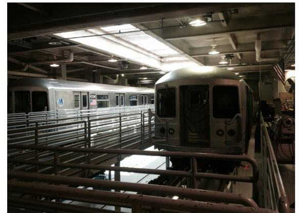
DCAS Fleet was invited to a CTE meeting and tour of the facility in April. The subway cars were donated by MTA in 2009, and brought into the school some distance away from the closest tracks through an elaborate towing and crane operation. Students are able to walk into and under the cars to conduct mechanical and electrical lab exercises on them.
